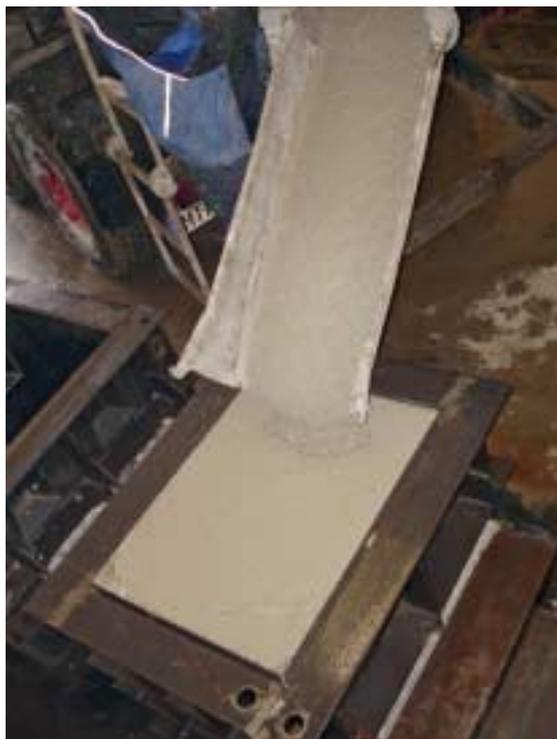
Fig. 8 Trial concreting UHPC.
